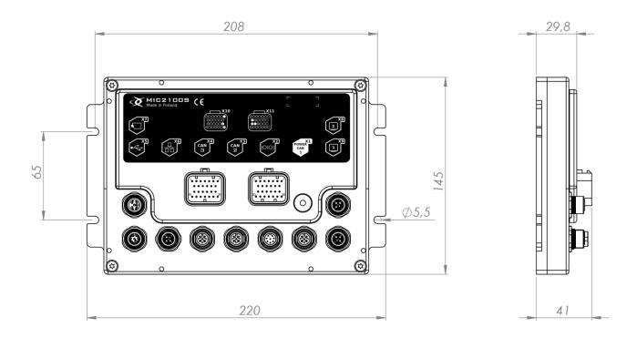
**Note!** Extra care should be paid on grounding of MIC2100S. It is recommended to use star lock washer under fastening bolt. Also, extra attention should be paid that lock washer goes through the paint layer.
