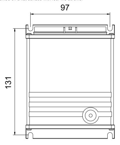
**NOTE!** Extra care should be paid on grounding of HCM2010S. It is recommended to use star lock washer under fastening bolt. Also, extra attention should be paid that lock washer goes through the paint layer.
