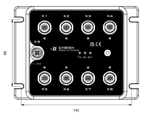
The preferred mounting position is connectors pointing downwards. If the unit is mounted connectors pointing to the side, then it is vital to leave some loose cable with a downward cue to prevent the ingress of moisture through connector.
