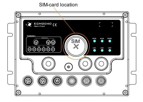
After opening the plug, the SIM card tray can be seen. First the metal cover must be opened.
