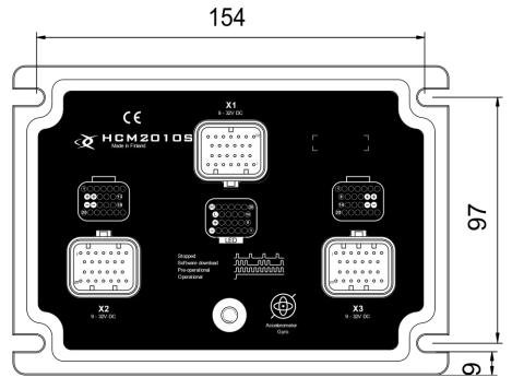
**NOTE!** Extra care should be paid on grounding of HCM2010S. It is recommended to use star lock washer under fastening bolt. Also, extra attention should be paid that lock washer goes through the paint layer.
