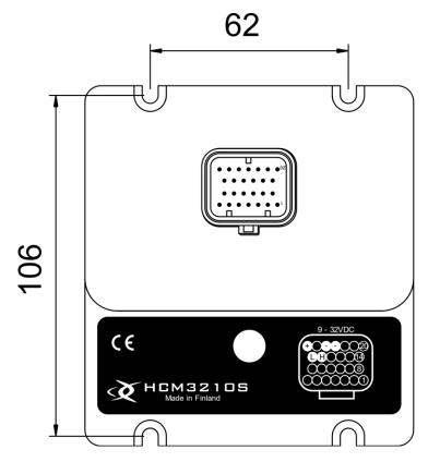
The preferred mounting position is connectors pointing downwards. If the unit is mounted connectors pointing to the side, then it is vital to leave some loose cable with a downward cue to prevent the ingress of moisture through connector.
