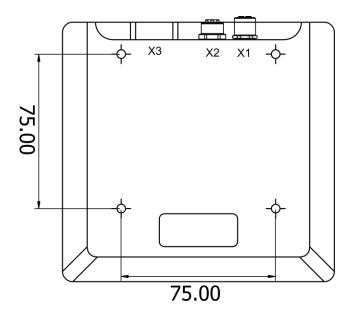
The preferred mounting position is connectors pointing downwards. If the unit is mounted connectors pointing to the side, then it is vital to leave some loose cable with a downward cue to prevent the ingress of moisture through connector.
